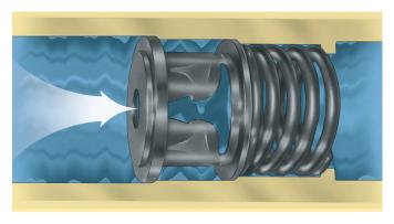
Now fully retracted, only the AutoFlow piston's end port is exposed. The regulator functions as a fixed orifice and will react to increased pressure differential with increased flow in
