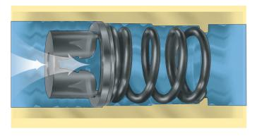
The differential pressure is below the minimum needed to activate the AutoFlow piston. It is fully extended and acts as a
