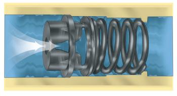
AutoFlow piston now responds to changes in differential pressure by repositioning the variable side orifices to maintain
