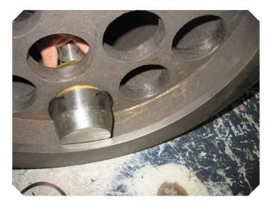
Pushing the tip of the spring into groove first.
