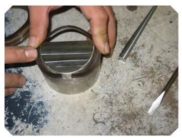
Place wave ring on tool with high side. The high side is shown in the picture when ends of spring are pointing up.
