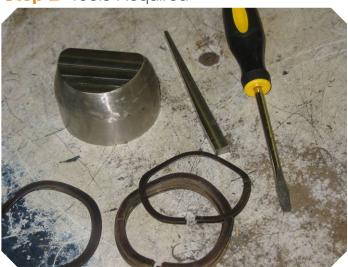
Flat screwdriver, spring insert adapter, no-go gauge.
