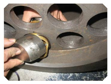
Remove the spring insert adapter out of the body.
