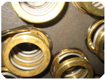
Place screwdiver on the gap and lift the spring out.
