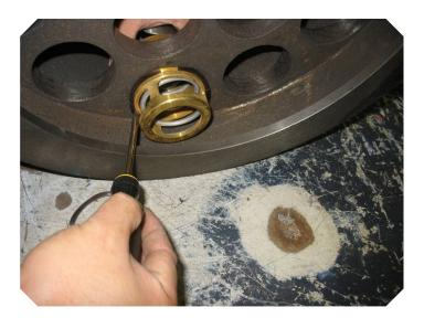
Use the flat screwdriver to push the spring into the groove.
