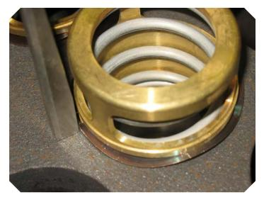
Wave spring is fitting correctly if the gauge doesnt go into gap as shown in picture above.
