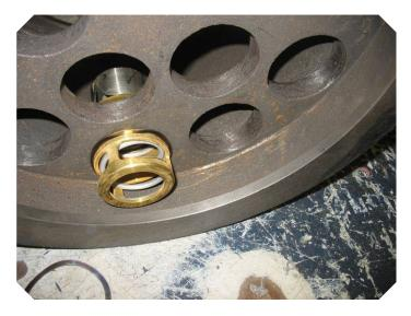
Wave spring is inserted within groove.
