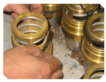
Insert gasket onto canister bottom.
