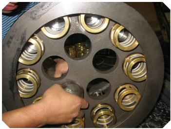
Insert tool with wave spring onto canister
